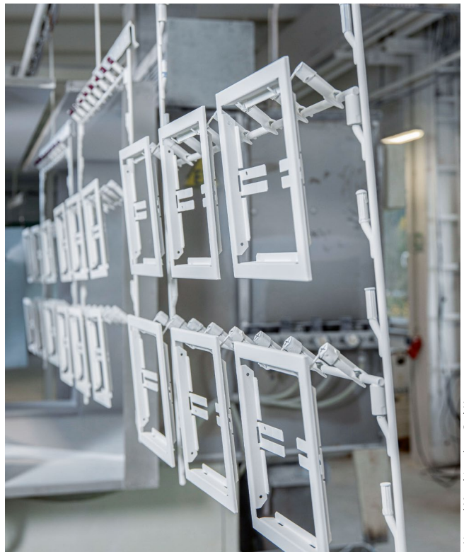
The finished coated workpieces.
