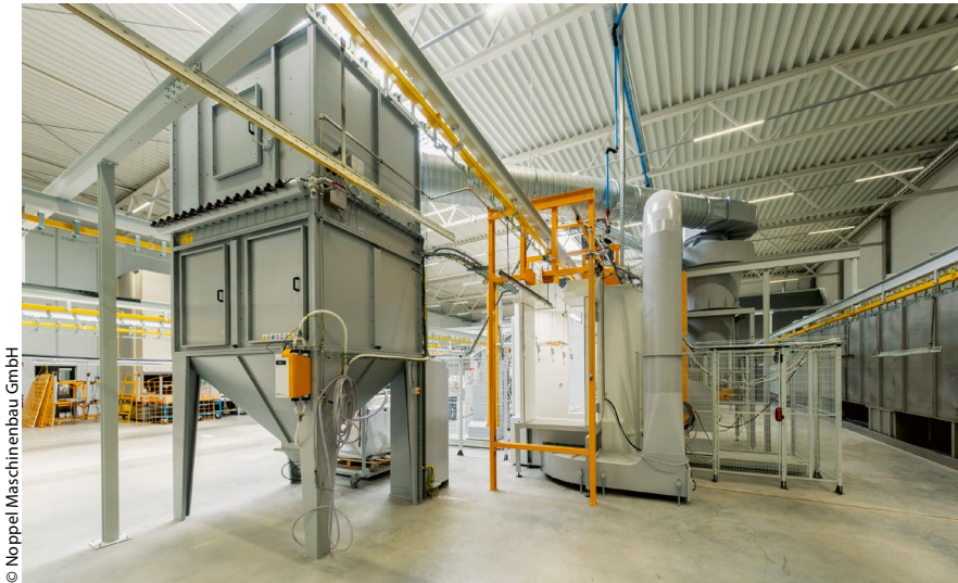
The modern powder booth for automatic operation features workpiece recognition and cyclone powder coating recovery as well as a large manual coater area.
