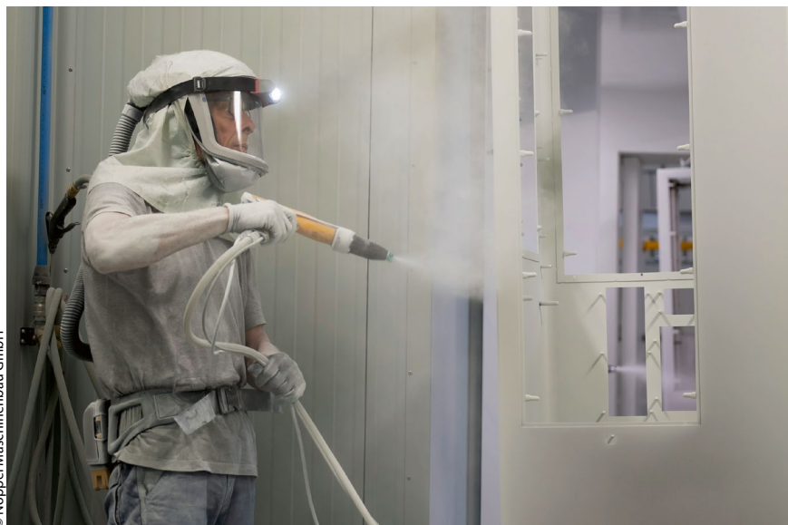
A separate manual powder booth for individual parts, small batches or for additional recoating of workpiece areas that are particularly difficult to access is also integrated into the system.
